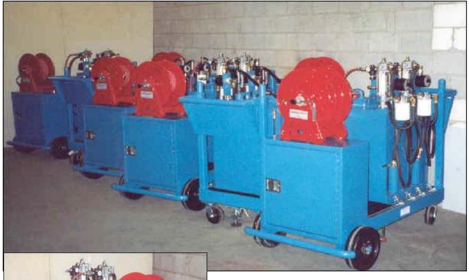
Portable Lube Carts to deliver maintenance lubricants and hydraulic fluids to reservoirs on the production machinery. Carts are modular in design to accommodate reservoir changes. Bothe air operated and manual pumps are used depending on the fluid and the requirements. Units have lockable cabinets for miscellaneous cleaning agents, tools, log book, etc. Flip up desk for manual record keeping.
